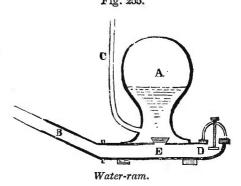
portion of water is driven into the reservoir as before, and so it repeatedly continues. The great force of the compressed air in the reservoir drives the water up the discharge-pipe, C, to any required height or distance.
