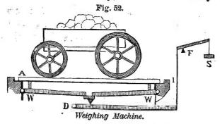
The wagon rests on the platform A (fig. 52,) and this platform rests on two levers at W, W, which presses their other ends both on a central point, and this again bears on
