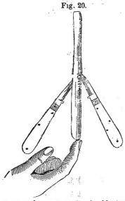
Centre of gravity maintained by two penknives.
