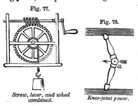
the levers is fixed to a solid beam, and the other connected with a movable block. When the joint a is forced in the direction indicated by the arrow, it produces a powerful pressure upon the movable block, which in-
