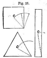
is narrow. For instance, the square block (fig. 26) is less easily thrown over than the tall and narrow block of equal weight, because, in turning the square block over its lower edge, the centre of gravity must be lifted up considerably in the curve shown by the dotted line c; but with a tall, narrow block, this curve being almost on a level, very little lifting is re-
