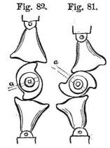
are at first near together, but are crowded asunder as the lever is pressed downward. This cheese-press is made of cast-iron, and has great power; to try it, weights were increased upon the lever, until the iron frame broke with a force equal to sixteen tons.
