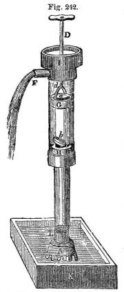
Common Pump: b, lower or fixed valve, G, piston with valve, a, opening upward; D d, pistonrod ; F, spout.
