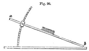
properties of the inclined plane, heretofore explained, that it requires a force equal to one-half the weight of the wooden block to slide it over a smooth wooden surface. Some kinds of wood have more friction than others, but this is about the average.\*
