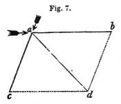
direction shown by the two arrows, and if one force be just sufficient to carry it from a to c, and the other to carry it from a to b, then it will move intermediate between the two, in the direction of the diagonal of the parallelogram a d, and to a dis-
