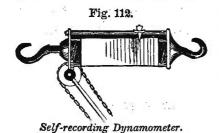
means of a wheel running on the ground, which gives motion to the roller through an endless chain, working a cogwheel by means of an endless screw. The cylindrical dynamometer, shown in fig. 112,
