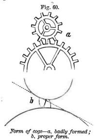
Liability of sliding is sometimes useful, by preventing the machinery from breaking when a sudden obstruction occurs. Where the force is great, the necessary tension or tightness of the cord produces too great a friction at the axle. In such cases, cogs or teeth must be resorted to.
