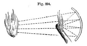
beating it out concave so as to fit a regularly curved gauge. If a foot in diameter, and carefully made, it will condense the rays of heat so powerfully at the focus, when held several feet from the fire, as to set fire to a pine stick or to flash gunpowder (fig. 294).
