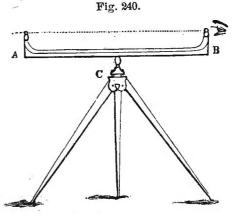
level, as shown by the air-bubble, by sighting through at the two wires, the levelness or descent of the land may be determined.
