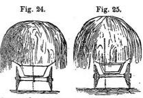
length, two tons may be piled upon the wagon with as much security from upsetting as one ton only on a short wagon.
