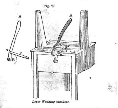
forated with holes, with great force against the clothes next to one side of the water-box. Like the printing-press, this machine exerts the greatest power just as the motion of the lever is completed, and at the time it is most needed. The same principle is exhibited in *Kendall's Cheese-press* (fig. 80), where the lever and the wheel and axle are combined with the two knee-joints, one on each side of the press, drawing down a cross-beam upon the cheese with a greatly multiplied power.
