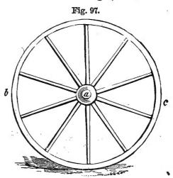
wheel will overcome twenty ounces of friction at the axle; or if the axle were twice as large, then, according to the same rule, it would require two ounces to overcome the same friction acting between larger surfaces.
