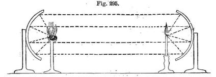
the dotted lines (fig. 295), and, setting fire to the phosphorus, will light the candle.
