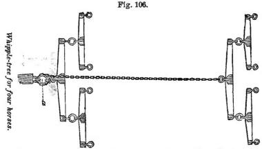
forward pair, by connecting the end of the chain at the same time to the plow.
