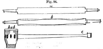
the outer ends, where they are soonest weakened by decay. Hence there should be nearly a uniform taper, slightly larger at the middle, and with an enlargement at the outer end, as c (fig. 94).
