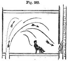
Hence the importance of Furnace and Open Fire-place Combined. the admission of currents of fresh air into all occupied rooms, by means of ventilation.
