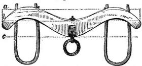
timber as wide as the dotted lines a c; and being thus weakened, it requires to be correspondingly large. Fig. 92 is equally strong, much lighter, and is easily made from a stick of timber only as wide as a b in the former figure.
