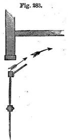
same good result may be reached by Window Ventilation. omitting the open fire-place and placing a register in the chimney at the floor, the ascending current in the chimney producing a constant draught through the register.
