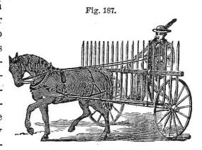
tached to a journal at the centre of the rake-head. By means of cams, stop, and spring, the lever and head are entirely at the will of the operator. A slight pressure, equal to seven or eight pounds, on a lever, causes the rake to revolve; and it is also readily elevated for backing, or for passing obstructions.
