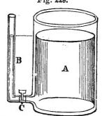
of the sides fourteen inches below the surface. If the tube, C, be an inch square, the water will be driven into it with a force of half a pound, and will press with that force against the one-inch surface of the stop-cock, C. If
