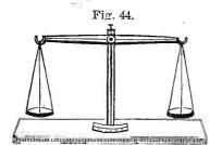
other, and on this its usefulness and accuracy entirely depend. The most sensitive balances have light beams with long arms, and the turning-point of hardened steel or agate, in the form of a thin wedge, on which the balance
