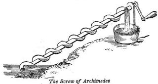
easily made by winding a lead tube around a wooden eylinder or rod (fig. 241), in the form of a screw.
