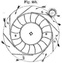
Section of Van de Water Wheel. buckets separate.
