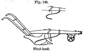
forms. Sometimes it is bent in the form of a bow with the lower point projecting forward, as in the upper figure; another form is like that shown in the lower cut, pointing backwards. This is less liable to be caught by obstructions. The weed-hook operates on the principle of bending the tall growth forward and prostrate, so that the turning sod completely buries it. The same object is
