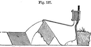
The Inclined Cutter, Laying Flat Furrows.
