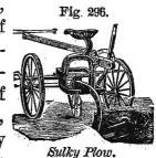
plowman rides, and controls, by means of levers at his hand, the depth and direction to the right or left.
