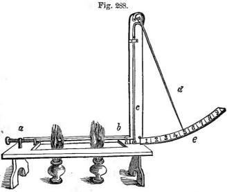
into the hole. The expansion may be more visibly shown and accurately measured by means of an instrument called the *Pyrometer* (fig. 288). The rod a b, secured to its
