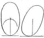
nearer the touching-point, that is, causes it to descend, and the body consequently falls over on its side. This may be easily illustrated with an egg, which will lie at rest upon its side, but falls when set on either end.
