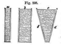
shape of the vessel may be. If, for instance, the vessel a (fig. 228), be one inch in diameter, and the vessel b be three inches in diameter, the water being equally high in both, the pressure on the whole bottom of b will be nine times as great as on
