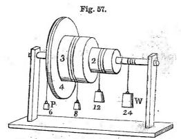
Wheel and axle, showing the heavier weight for less motion.
