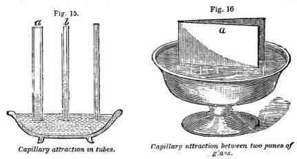
two small plates of glass, placed with their edges in war ter, in contact on one side, and a little open at the other side, as in fig. 16. As the faces of the plates approach each other, the water rises higher, forming the curve,  $\alpha$ .
