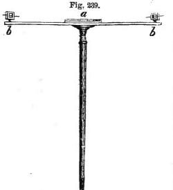
lowing manner:—Procure a mason's or carpenter's spirit-level, (a. fig. 239) fasten it to the upper side of a straight bar of wood, and on the ends of this bar secure small, upright pieces of tin plate, b, b, having openings cut in the Horizontally centre. across these openings, draw very fine wire, which shall be exactly at equal heights above
