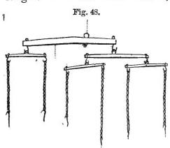
worked abreast, the two horses placed together should have only half the length of arm of the main whiffle-tree as the single horse, fig. 48. The farmer who has a team of two horses unlike in strength, may thus easily know how to adjust the arms of the
