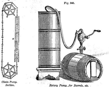
here shown, (fig. 247), the chain is made to revolve rapidly on the angular wheel by means of a winch attached to
