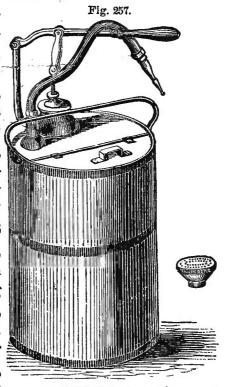
and in a neat and compact Culindrical Garden-engine. form, the working part being within the cylindrical case.
