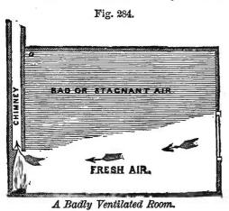
warmed with a stove or open fire-place, the entrance should be near the ceiling above. If over the window, with a narrow, sloping board to throw the current upwards as in fig. 283, the fresh air will be distributed through the room, and will descend towards
