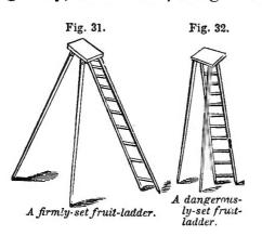
its legs more widely spread, to be secure from falling, than if the centre were lower down. Hence such a position, as in fig. 32, would be unsafe.
