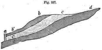
rain falls upon the surface, as at c d, it sinks down in the more porous parts between these layers, to c. If the layers happen to be broken in any place below, the water finds its way up through the crevices by the pressure of the head above, and forms springs. If there are no openings through the rocks, deep borings are sometimes made
