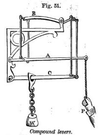
A, exerting a force on the lever B five times as great as the power. B acts on the lever C with a force increased three times, and this, again, on the weight, W, with a four-fold force. Multiplying 5, 3, and 4 together, the product is 60; hence a force of one pound at P will support 60 pounds at W. By gradumarking ating (or notches) the lever C, so that the distance is measured as
