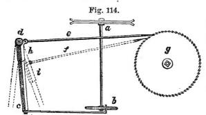
stated. In doing so, it causes the arm d c, to vibrate backwards and forwards, on a pin at d; the connecting rod b c being set near the circumference
