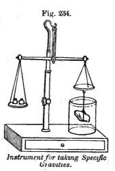
It was in a similar way that Archimedes is said to have succeeded in detecting the suspected fraud in the manufacture of the golden crown of the ancient king of Syracuse. He first weighed it, and then found that it displaced more water when plunged in a vessel just filled than a piece of pure gold, and also that it displaced less than silver, whence he inferred the mixture of these two metals.
