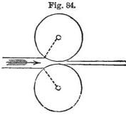
Principle of the knee-joint in the rolling-mill
